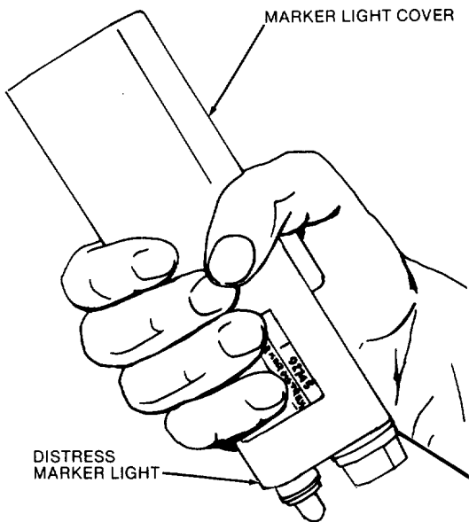
Figure 4. Distress Marker Light with Flashguard
